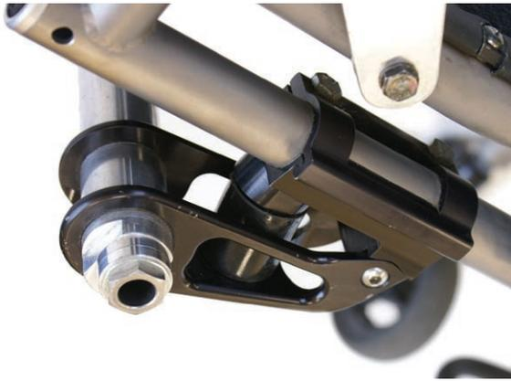
Suspension arm attached to frame and camber bar
